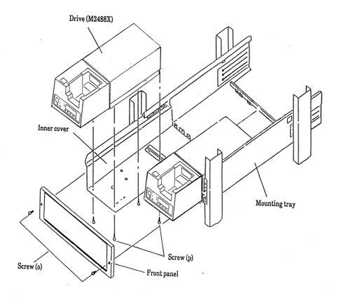
Figure 1-17. M2488 with ACL Tray Mounting
